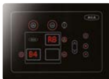
Capacitance touch-screen control
